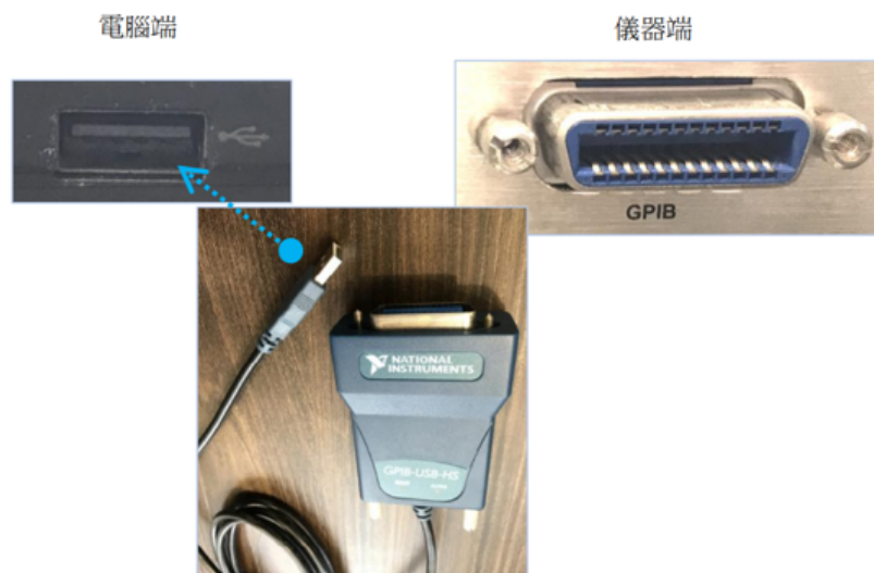
Figure1. GPIB interface connects to the instrument
